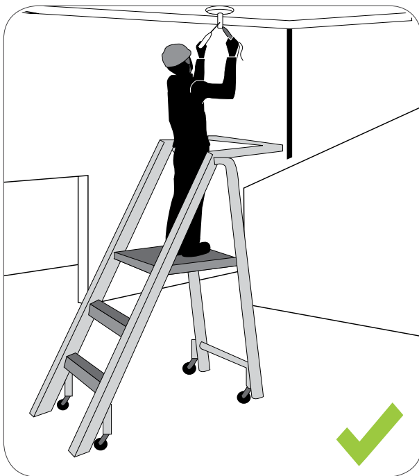
Figure 11.2: A step platform can provide a more stable work surface.
