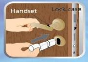
2. Insert the cylinder into the lock case till you are able to turn the locking cam.
