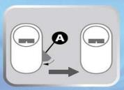
Turn locking cam **A** with knob to align with the cylinder.
