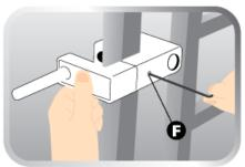
6. From outside of the gate, position your lock to desired height and secure it by tightening the locking screw in hole F.
