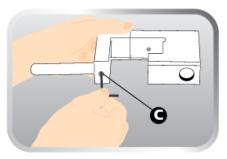
2. Align hole B with hole C. Insert Allen Key and turn anti-clockwise to loosen internal locking screw.
