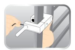
5. Align hole **B** with hole **C**, tighten internal locking screw in clockwise direction with Allen Key.
