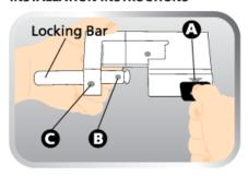
1. Insert Key into keyhole A. Turn Key clockwise to release the locking bar.
