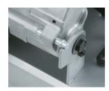
Change of saw head locking device from chain lock to pin lock (LW1400 only)
