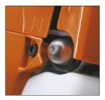
**Inertia chain brake** Effective inertia-activated chain
