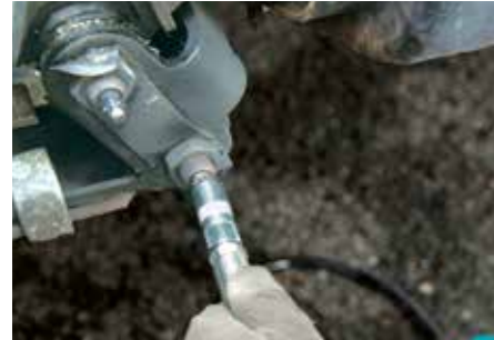
Flexible hose with adapter Length: 1200mm Standard equipment Part No. 191A79-9
